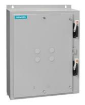
Duplex starter w/o alternator, Size 0, Three phase full voltage, Solid-state overload relay, OLR amp range 3-12A, 380-440/440-480V 50/60Hz coil, Combination type, Two 10A circuit breakers, Enclosure NEMA type 1, Indoor general purpose use
