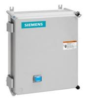
Non-reversing motor starter, Size 1 3/4, Three phase full voltage, Solid-state overload relay, OLR amp range 10-40A, Non-combination type, Enclosure type 4X fiberglass, Water/dust tight noncorrosive, Standard width enclosure
