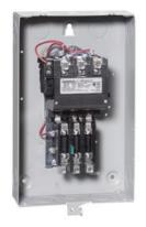
Non-reversing motor starter, Size 2 1/2, Three phase full voltage, Amb. compensate bimetal OLR, Contactor amp rating 60A, Non-combination type, Enclosure type 1, Indoor general purpose use
