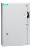
Reversing motor starter, Size 3, Three phase full voltage, Solid-state overload relay, OLR amp range 25-100A, 110V 50Hz / 120V 60Hz coil, Combination type, 100A disconnect switch, Enclosure NEMA type 1, Indoor general purpose use
