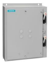
Duplex starter w/ alternator, Size 0, Three phase full voltage, Solid-state overload relay, OLR amp range 3-12A, 110V 50Hz / 120V 60Hz coil, Combination type, Two 10A circuit breakers, Enc NEMA type 4 painted steel, Water/dust tight for outdoors
