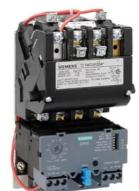
Non-reversing motor starter Size 0 Single phase full voltage Solid-state overload relay OLRelay amp range 5.5-22A 110-120/220-240VAC 60HZ coil Combination type No enclosure
