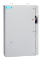
Non-reversing motor starter Size 1 Three phase full voltage Solid-state overload relay OLRelay amp range 10-40a 380-440/440-480V 50/60HZ coil Combination type 30Amp circuit breaker Encl NEMA type 4X 316 S-steel Water/dust tight noncorrosive Extra-wide enclosure
