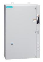
Non-reversing motor starter, Size 3, Three phase full voltage, Solid-state overload relay, OLR amp range 25-100A, Combination type, 100A non-fusible disconnect, Enclosure NEMA type 4/12, Water/dust tight for outdoors, Standard width enclosure
