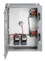
Pump control panel, Duplex controller NEMA size 3 Solid-state overload relay, OLR amp range 25-100A, 120 VAC coil, Fusible disconnect HOA Sel Sw. and Start P.B., Enclosure NEMA type 3/3R,12 Weather proof outdoor use
