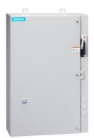
Non-reversing motor starter, Size 2 1/2, Three phase full voltage, Solid-state overload relay, OLR amp range 25-100A, 240V 50Hz / 277V 60Hz coil, Combination type, 100A circuit breaker, Encl NEMA type 4X 316 S-Steel, Water/dust tight noncorrosive, Standard width enclosure
