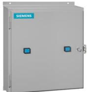
Duplex starter w/o alternator, Size 4, Three phase full voltage, Solid-state overload relay, OLR amp range 50-200A, 380-440/440-480V 50/60Hz coil, Non-combination type, Enclosure NEMA type 12, Dust/drip proof for indoors
