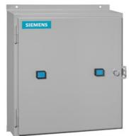
Duplex starter w/o alternator, Size 1, Three phase full voltage, Solid-state overload relay, OLR amp range 10-40A, 380-440/440-480V 50/60Hz coil, Non-combination type, Encl NEMA type 4X 304 S-Steel, Water/dust tight noncorrosive
