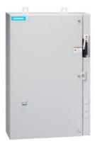
Non-reversing motor starter, Size 2, Three phase full voltage, Solid-state overload relay, OLR amp range 13-52A, Combination type, 60A non-fusible disconnect, Encl NEMA type 4X 304 S-Steel, Water/dust tight noncorrosive, Extra-wide enclosure
