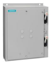
Duplex starter w/ alternator, Size 3 1/2, Three phase full voltage, Solid-state overload relay, OLR amp range 50-200A, 110V 50Hz / 120V 60Hz coil, Combination type, Two 125A circuit breakers, Enclosure NEMA type 1, Indoor general purpose use
