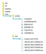
Figure 8-1 File structure of the IOP2
