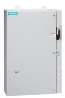
Non-reversing motor starter, Size 1, Three phase full voltage, Solid-state overload relay, OLR amp range 3-12A, Combination type, 30A non-fusible disconnect, Encl NEMA type 4X 304 S-Steel, Water/dust tight noncorrosive, Extra-wide enclosure
