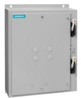
Duplex starter w/o alternator, Size 1 3/4, Three phase full voltage, Solid-state overload relay, OLR amp range 10-40A, 240V 50Hz / 277V 60Hz coil, Combination type, Two 40A circuit breakers, Encl NEMA type 4X 304 S-Steel, Water/dust tight noncorrosive
