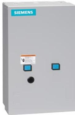
2-speed 3-phase motor starter. Size 0, Two separate windings, Constant or variable torque, Solid-state overload relays, Low Spd OLR range 0.75-3.4A, High Spd OLR range 0.75-3.4A, Enclosure NEMA type 1, Indoor general purpose use
