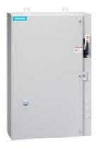
Non-reversing motor starter, Size 1, Three phase full voltage, Solid-state overload relay, OLR amp range 3-12A, Combination type, 30A fusible disconnect, 30A/250V fuse clip, Encl NEMA type 4X 304 S-Steel, Water/dust tight noncorrosive, Extrawide enclosure
