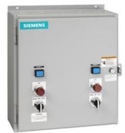
Duplex starter w/ alternator, Size 0, Three phase full voltage, Solid-state overload relay, OLR amp range 5.5-22A, 110V 50Hz / 120V 60Hz coil, Non-combination type, Encl NEMA type 4X 304 S-Steel, Water/dust tight noncorrosive
