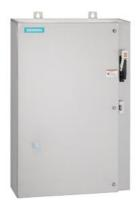
Non-reversing motor starter Size 1 Three phase full voltage Solid-state overload relay OLRelay amp range 0.25-1A 208VAC 60HZ coil Combination type 30Amp non-fusible disconnect Encl NEMA type 4X 316 S-steel Water/dust tight non-corrosive Extra-wide enclosure
