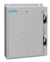
Duplex starter w/o alternator, Size 0, Three phase full voltage, Solid-state overload relay, OLR amp range 5.5-22A, 190-220/220-240V 50/60Hz coil, Combination type, Two 25A circuit breakers, Enclosure NEMA type 12, Dust/drip proof for indoors
