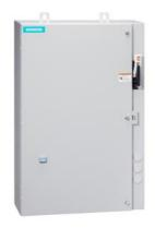
Non-reversing motor starter, Size 2 1/2, Three phase full voltage, Solid-state overload relay, OLR amp range 25-100A, Combination type, 100A circuit breaker, Encl NEMA type 4X 304 S-Steel, Water/dust tight noncorrosive, Standard width enclosure
