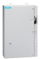
Non-reversing motor starter Size 0 Three phase full voltage Solid-state overload relay OLRelay amp range 3-12A 380-440/440-480V 50/60HZ coil Combination type 10Amp circuit breaker Encl NEMA type 4X 316 S-steel Water/dust tight noncorrosive Extra-wide enclosure
