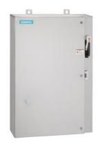
Non-reversing motor starter, Size 3, Three phase full voltage, Solid-state overload relay, OLR amp range 25-100A, Combination type, 100A fusible disconnect, 100A/250V fuse clip, Encl NEMA type 4X 304 S-Steel, Water/dust tight noncorrosive, Extra-wide enclosure
