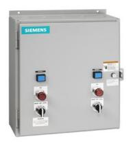
Duplex starter w/ alternator, Size 0, Three phase full voltage, Solid-state overload relay, OLR amp range 0.25-1A, 110V 50Hz / 120V 60Hz coil, Non-combination type, Encl NEMA type 4X 304 S-Steel, Water/dust tight noncorrosive
