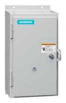
Non-reversing motor starter, Size 2 1/2, Three phase full voltage, Solid-state overload relay, OLR amp range 25-100A, 110V 50Hz / 120V 60Hz coil, Non-combination type, Enclosure type 12, Dust/drip proof for indoors, Standard width enclosure
