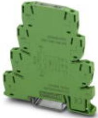
PLC-INTERFACE as an electronic reversing load relay, consisting of PLC-BSP.../21 basic terminal block with spring-cage connection and integrated circuit, for driving DC motors, with LED and protective circuit, output: 10 ... 30 V DC/2 A
