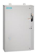
Non-reversing motor starter, Size 2 1/2, Three phase full voltage, Solid-state overload relay, OLR amp range 25-100A, Combination type, 100A circuit breaker, Encl NEMA type 4X 304 S-Steel, Water/dust tight noncorrosive, Extra-wide enclosure
