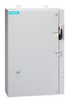
Non-reversing motor starter Size 3 Three phase full voltage Solid-state overload relay OLRelay amp range 25-100A 380-440/440-480V 50/60HZ coil Combination type 125Amp circuit breaker Enclosure NEMA type 4/12 Water/dust tight for outdoors Standard width enclosure
