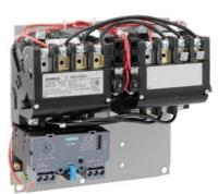
Reversing motor starter Size 1 Three phase full voltage Solid-state overload relay OLRelay amp range 0.25-1A 208VAC 60HZ coil Non-combination type Enclosure type (open)
