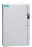
Non-reversing motor starter Size 1 Three phase full voltage Solid-state overload relay OLRelay amp range 0.75-3.4A 190-220/220-240V 50/60HZ coil Combination type 3Amp circuit breaker Encl NEMA type 4X 316 S-steel Water/dust tight noncorrosive Extra-wide enclosure
