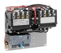
Reversing motor starter Size 1 Three phase full voltage Solid-state overload relay OLRelay amp range 0.25-1A 380-440/440-480V 50/60HZ coil Non-combination type Enclosure type (open)
