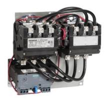
Reversing motor starter Size 4 Three phase full voltage Solid-state overload relay OLRelay amp range 50-200A 220-240/440-480VAC 60HZ coil Non-combination type Enclosure type (open)
