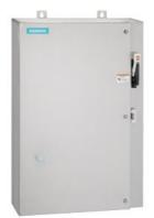
Non-reversing motor starter Size 1 Three phase full voltage Solid-state overload relay OLRelay amp range 10-40a Combination type 60Amp non-fused disconnect Encl NEMA type 4X 316 S-steel Water/dust tight non-corrosive Extra-wide enclosure
