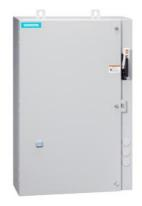
Non-reversing motor starter, Size 2, Three phase full voltage, Solid-state overload relay, OLR amp range 13-52A, 24VAC 50-60Hz coil, Combination type, 50A circuit breaker, Encl NEMA type 4X 304 S-Steel, Water/dust tight noncorrosive, Extrawide enclosure
