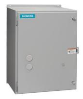
Reversing motor starter, Size 4, Three phase full voltage, Solid-state overload relay, OLR amp range 50-200A, 110 120/220 240VAC 60Hz coil, Non-combination type, Enclosure type 12, Dust/drip proof for indoors, Standard width enclosure
