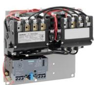
Reversing motor starter Size 1 Three phase full voltage Solid-state overload relay OLRelay amp range 3-12A 110-120/220-240VAC 60HZ coil Non-combination type Enclosure type (open)
