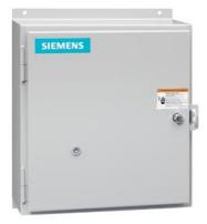
Reversing motor starter, Size 2, Three phase full voltage, Solid-state overload relay, OLR amp range 13-52A, Non-combination type, Enclosure type 12, Dust/drip proof for indoors, Standard width enclosure
