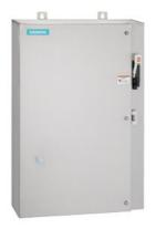
Non-reversing motor starter Size 0 Three phase full voltage Solid-state overload relay OLRelay amp range 5.5-22A 208VAC 60HZ coil Combination type 30Amp non-fusible disconnect Encl NEMA type 4X 316 S-steel Water/dust tight non-corrosive Extra-wide enclosure
