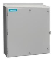
Non-reversing motor starter, Size 4, Three phase full voltage, Solid-state overload relay, OLR amp range 50-200A, 208VAC 60Hz coil, Non-combination type, Enclosure type 12, Dust/drip proof for indoors, Standard width enclosure
