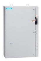
Non-reversing motor starter, Size 2 1/2, Three phase full voltage, Solid-state overload relay, OLR amp range 25-100A, 208VAC 60Hz coil, Combination type, 100A fusible disconnect, 100A/600V fuse clip, Encl NEMA type 4X 304 S-Steel, Water/dust tight noncorrosive, Standard width enclosure
