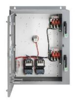
Pump control panel, Duplex controller NEMA size 1 Solid-state overload relay, OLR amp range 5.5-22A, 120 VAC coil, Fusible disconnect HOA Sel Sw. and Start P.B., Enclosure NEMA type 3/3R,12 Weather proof outdoor use
