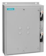
Duplex starter w/o alternator, Size 3, Three phase full voltage, Solid-state overload relay, OLR amp range 25-100A, 380-440/440-480V 50/60Hz coil, Combination type, Two 100A circuit breakers, Enc NEMA type 4 painted steel, Water/dust tight for outdoors
