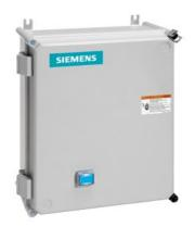
Non-reversing motor starter, Size 4, Three phase full voltage, Solid-state overload relay, OLR amp range 50-200A, 208VAC 60Hz coil, Non-combination type, Enclosure type 4X fiberglass, Water/dust tight noncorrosive, Standard width enclosure
