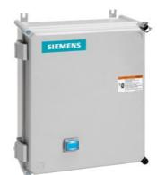
Non-reversing motor starter, Size 1, Three phase full voltage, Solid-state overload relay, OLR amp range 0.75-3.4A, Non-combination type, Enclosure type 4X fiberglass, Water/dust tight noncorrosive, Standard width enclosure
