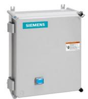
Non-reversing motor starter, Size 1 3/4, Three phase full voltage, Solid-state overload relay, OLR amp range 10-40A, 24VAC 50-60Hz coil, Non-combination type, Enclosure type 4X fiberglass, Water/dust tight noncorrosive, Standard width enclosure
