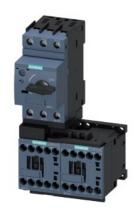
FUSELESS LOAD FEEDER REVERSING OPERATION, AC 400V, S00 0.7. . . . 1A, AC 110/120V 50/60HZ SCREW TERMINAL FOR RAIL MOUNTING, TYPE OF ASSIGNMENT 2, IQ = 150KA (ALSO FULFILLS TYPE OF ASSIGNMENT 1) 1NC (CONTACTOR)
