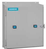
Duplex starter w/o alternator, Size 4, Three phase full voltage, Solid-state overload relay, OLR amp range 50-200A, 24VAC 50-60Hz coil, Non-combination type, Enc NEMA type 4 painted steel, Water/dust tight for outdoors
