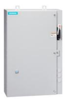
Non-reversing motor starter, Size 1, Three phase full voltage, Solid-state overload relay, OLR amp range 5.5-22A, Combination type, 30A non-fusible disconnect, Encl NEMA type 4X 304 S-Steel, Water/dust tight noncorrosive, Extra-wide enclosure
